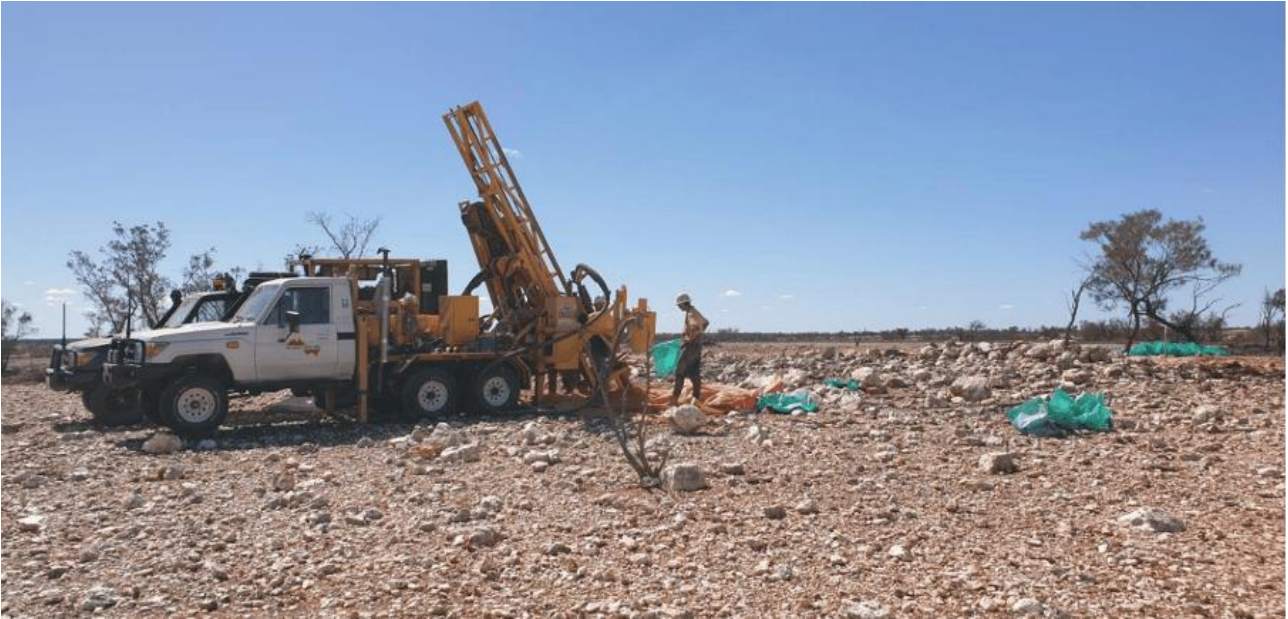
An aircore drill rig at the Bellagio Gold Prospect. Source: Supplied (KNB).
