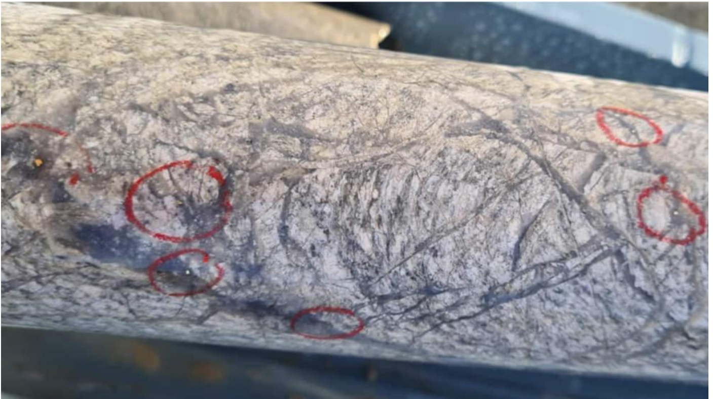
Visible gold (circled in red) in the 25ENDD001 drill core. Pic: Koonenberry Gold
