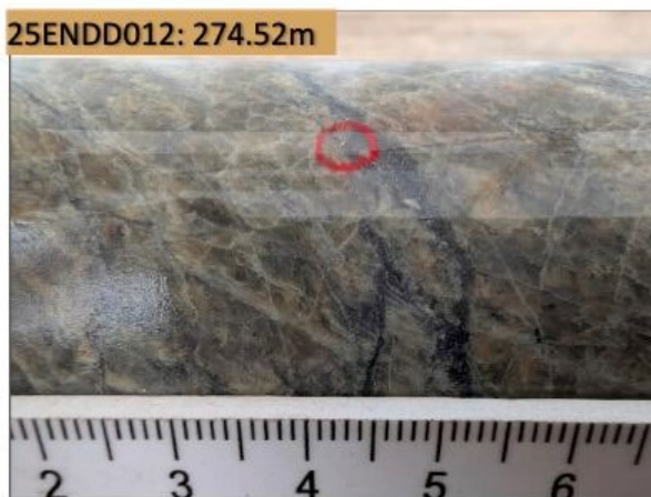
Photo 3. Visible gold (circled red) in hole 25ENDD012 at 274.52m down hole in carbonate-quartz-pyrite-arsenian pyrite vein within strongly phyllic altered granite host rock. Scale bar units are centimetres.
